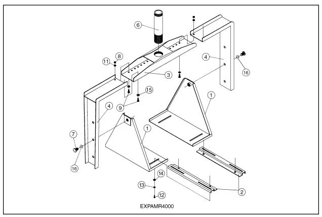
Figure 2. MR4000 Exploded Assembly
